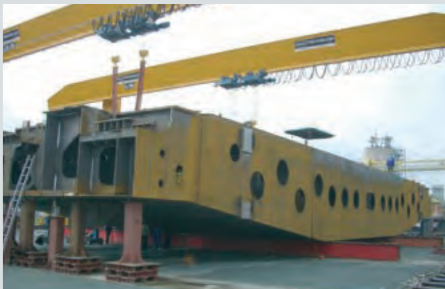
Fertigung Torsegmente - Manufacturing Gatesection
